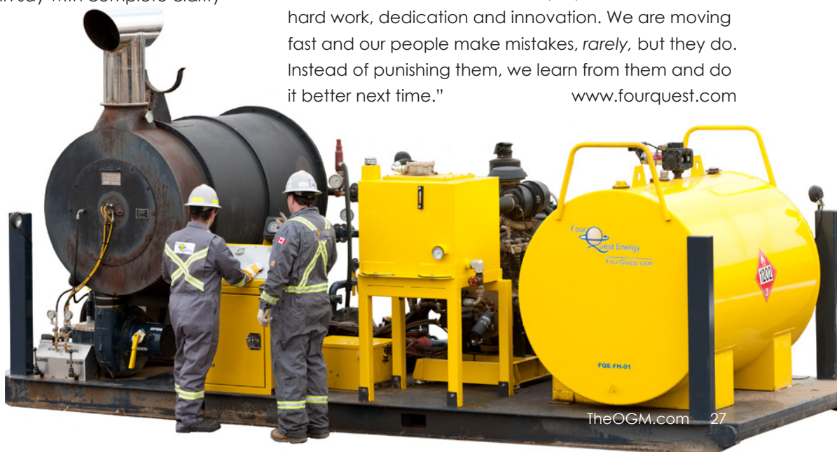
Carrying out water-heating operations with a 8 Million BTU inline heater.
