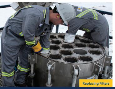
FourQuest Energy provides a large range of fluid filtration services, from ensuring particulate is filtered out of testing water to providing reverse osmosis filtration for boiler feed water.
