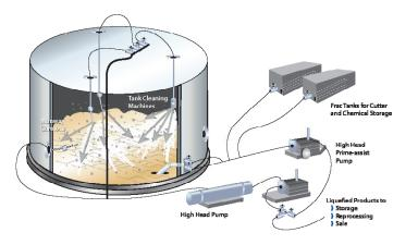
FourQuest Energy delivers a tank cleaning methodology that's tailormade to each vessel or tank - changing the industry standard as well as enhanced mechanical cleaning.
