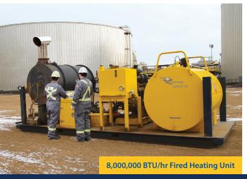
The FourQuest Energy fired heating units are coupled with a shell and tube heat exchanger using glycol as a heating medium. This allows us to heat corrosive and severe chemicals and liquids without any worry. The unit is specifically designed to safely heat most liquids. Our fired heating units have a thermal output of 8,000,000 BTU/hr and a maximum flow rate capacity of 500 L/min at 150 psig discharge pressure.
