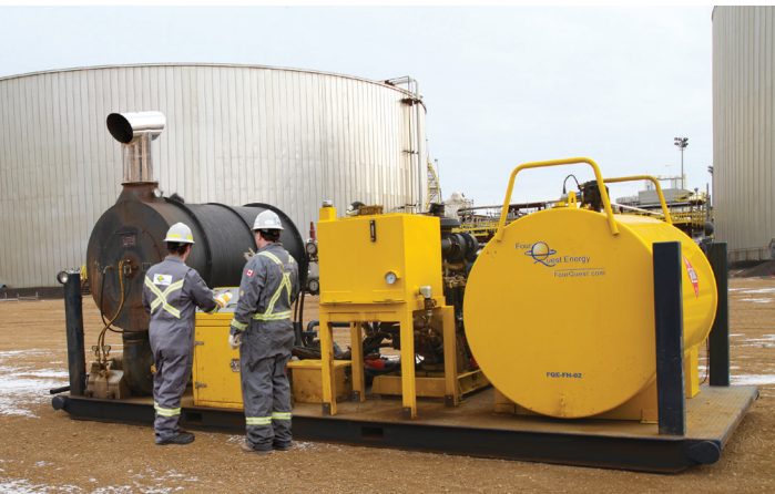
8,000,000 BTU/hr Fired Heating Unit
